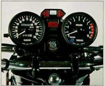
The instrumentation is the most complete, and the most logical, you are likely to find. A warning light even tells when a headlight filament has burned out. Unique, self-cancelling turn signals are standard.
