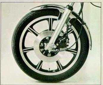
The attractive one-piece cast aluminum wheels eliminate tedious spoke tightening and wobble in the rims.
