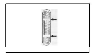
If a tire tread shows crosswise lines, it means that the tire is worn to its limit. Replace the tire.
