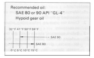
If desired, an SAE 80W/90 hypoid gear oil may be used for all conditions.
